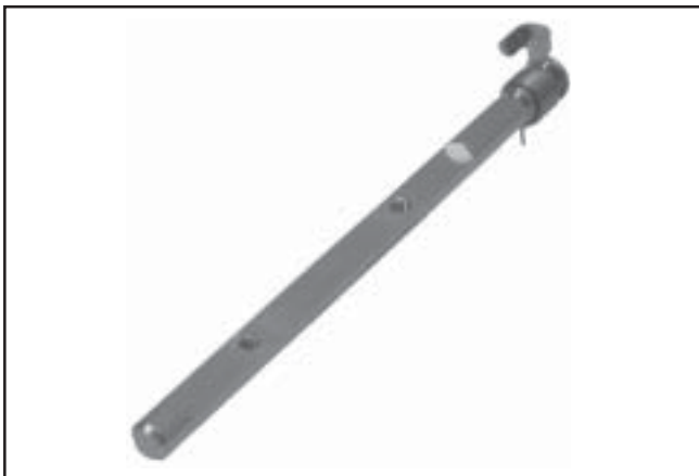
Figure 5-63. Choke Shaft and Spring Details.
